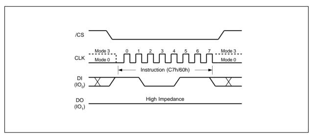
Figure 34. Chip Erase Instruction Sequence Diagram
