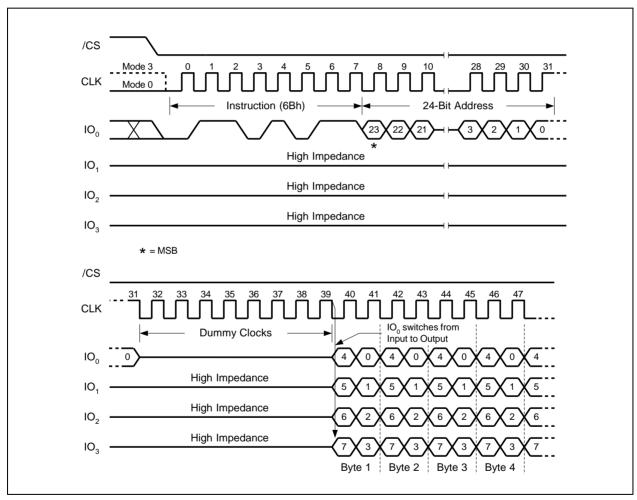
Figure 20. Fast Read Quad Output Instruction
