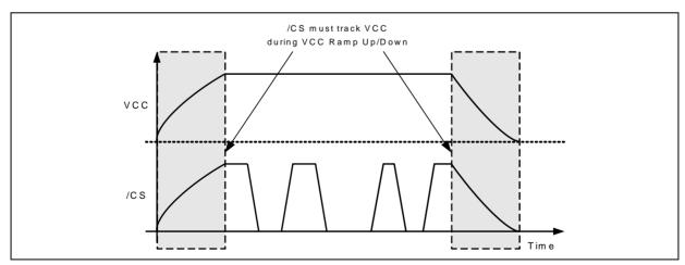
Figure 58b. Power-up, Power-Down Requirement
