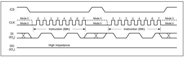
Figure 58a, Enable Reset and Reset Instruction Sequence
