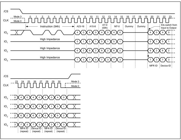
Figure 41. Read Manufacturer / Device ID Quad I/O Instruction
