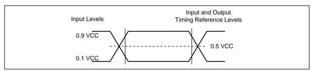
Figure 59. AC Measurement I/O Waveform
